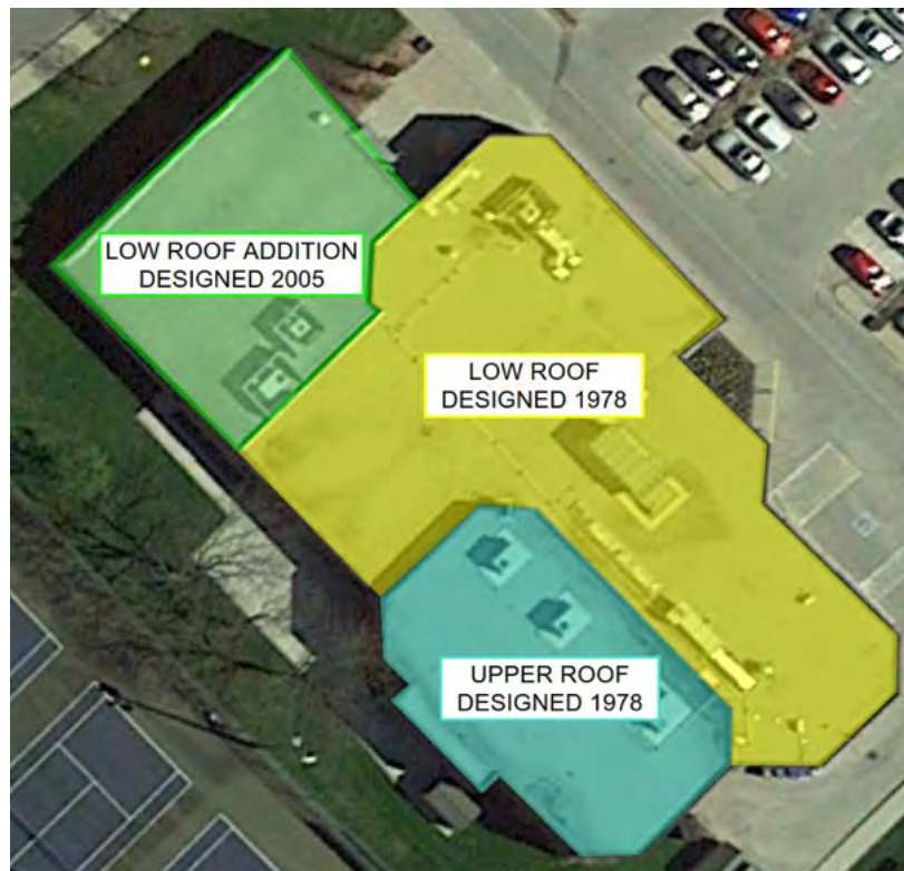
Figure 1: Burlington Seniors Centre roof areas.
